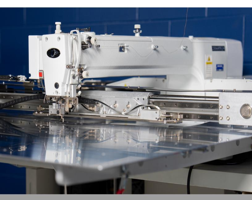
Dematron's DM-6055 is a high-performance computerized sewing machine with a 600 mm x 550 mm capacity, featuring powerful servo motors that enhance efficiency and precision, making it ideal for complex patterns and reducing labor costs across various applications.
