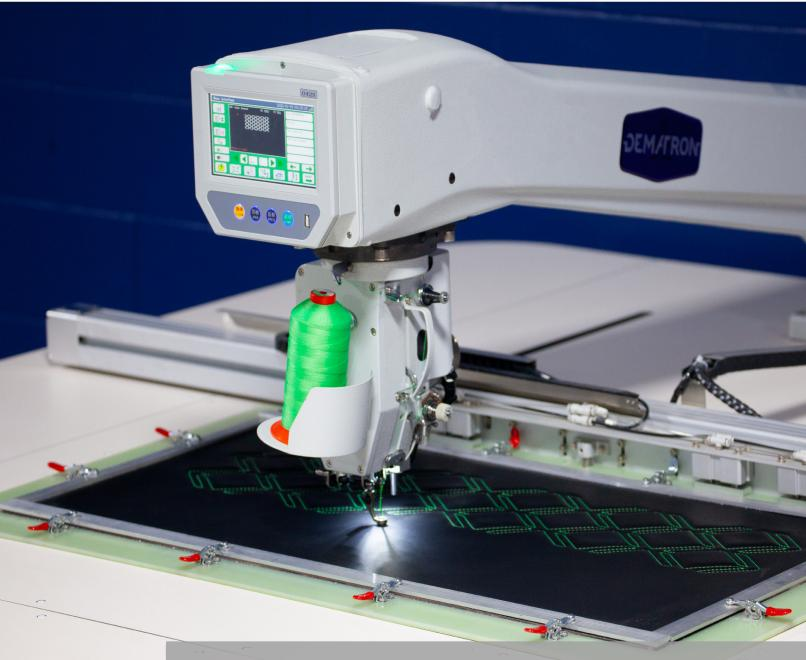
The Dematron XZ-1390 offers turning head capability and the largest CNC sew range while delivering unmatched quality and consistency. Ideal for intricate sewing sequences, decorative pattern quilting, part attachment and multi-piece sewing.
