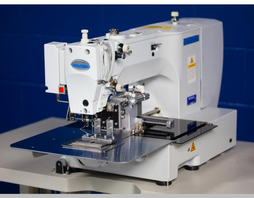
The Dematron DM-1010 offers 3.96" x 3.96" sew area and is able to handle a wide range of fabrics and materials suitable for various applications.
